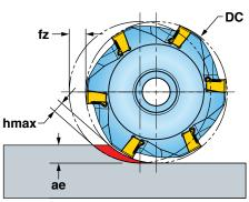
\* When ae is less than 25% DC, recommend use of Chip Thinning Calculator to ensure hmax falls within fz range.
